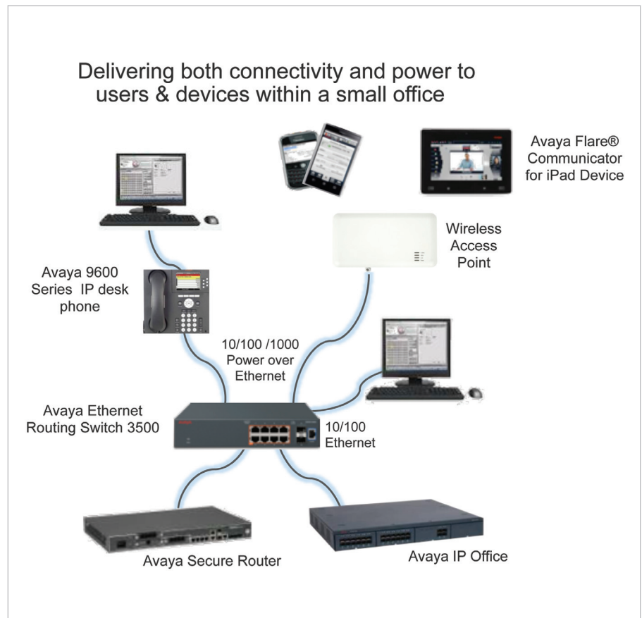
Figure 3: ERS 3500 deployment scenario
