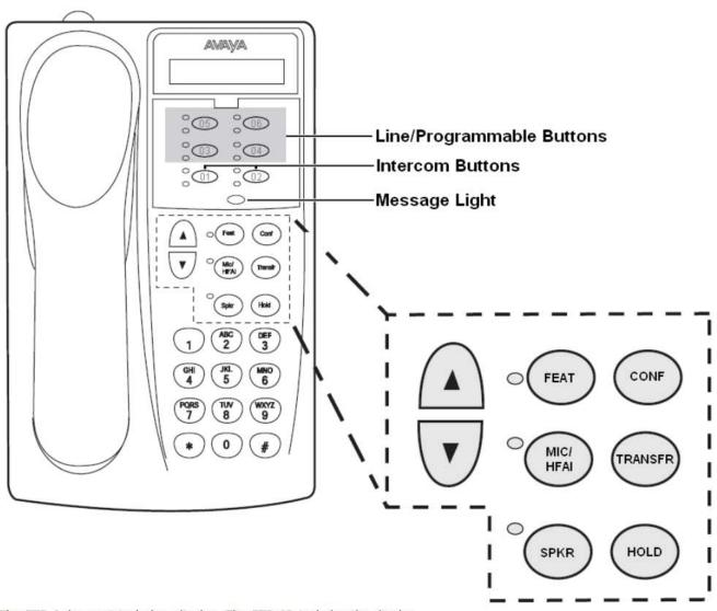
The ETR 6 does not include a display. The ETR 6D includes the display.
