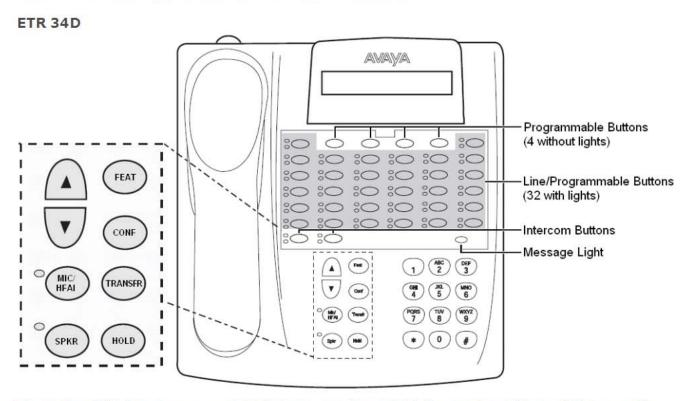
The number of ETR 34D phones supported is limited to a maximum of 4 (with a maximum of 2 per ETR6 base card).
