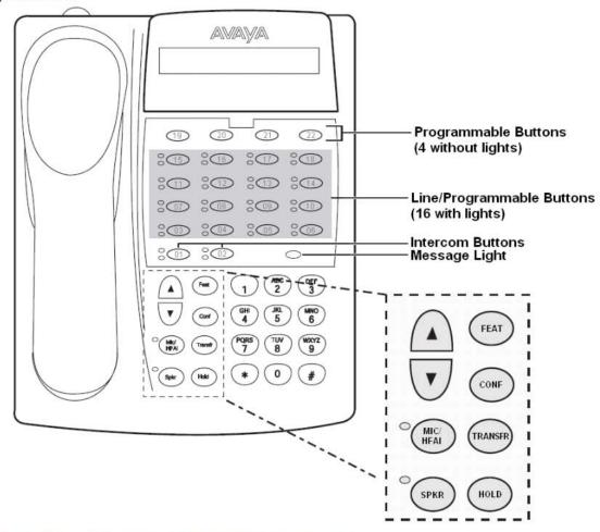
The ETR 18 does not include a display. The ETR 18D includes the display.
